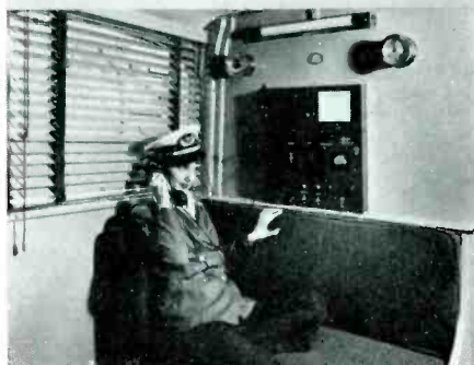
The "Revere" during a stopover in New York on her way South. Ultra modern in detail this 45-foot cruiser is made entirely of cupro-nickel welded to form a one-piece, seamless construction. Typical of her appointments is the Hallicrafters HT-12 Radiophone, bulkhead mounted in the main cabin. By this means boat-to-boat and boat-to-shore communication is provided over ranges up to several hundred miles
